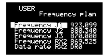
Move through the parameters list – the 'Up' / 'Down' buttons, parameter choice – the 'Right' / 'Left' buttons, edit choosing value – the 'Up' / 'Down' buttons
