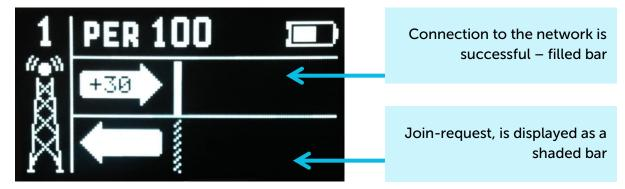
A shaded bar appears on the DM diagram if a failed attempt is made also. In total, the network tester takes three attempts to join the network.
