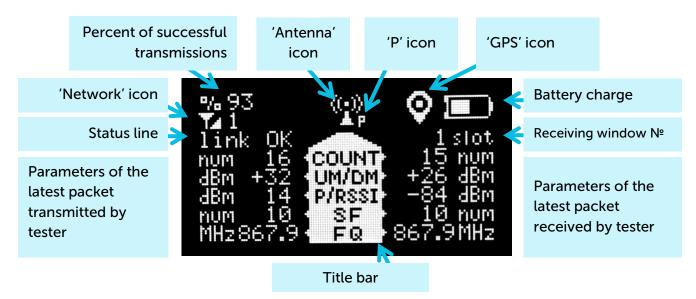
Unlike other screens, the work screen 2 displays information only about the last communication session. The accumulated data here is the PER coefficient and the total number of received / transmitted packets.
