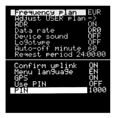
Frequency plan – choice of the frequency standard. EUR – European frequency plan. RUS – Russian frequency plan. USER – custom frequency plan.
