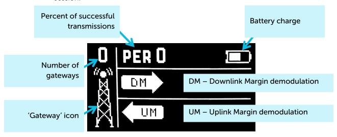
Margin demodulation is the positive integer value displayed in dBm and indicating how much received signal above the demodulation threshold. '0' value means that the packet was received on the bottom of demodulation (0 dBm), whereas, for example, '20' value means that the packet was received on 20 dBm above the demodulation threshold.
